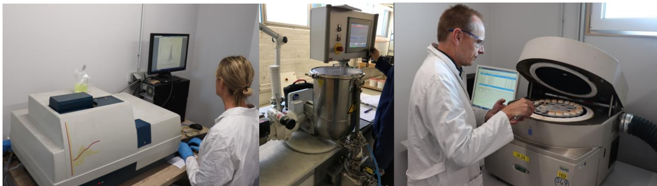
Figure: German Piloting Equipment (L - R) Laser Particle Sizer, Micronising Mill and Thermo Gravimetric Analyser
