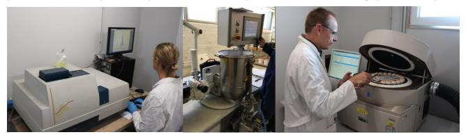
Figure: German Piloting Equipment (L - R) Laser Particle Sizer, Micronising Mill and Thermo Gravimetric Analyser
