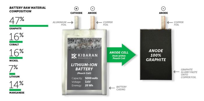
Figure 3: Lithium-ion Battery (Pouch Cell) showing raw material composition and graphite anode
