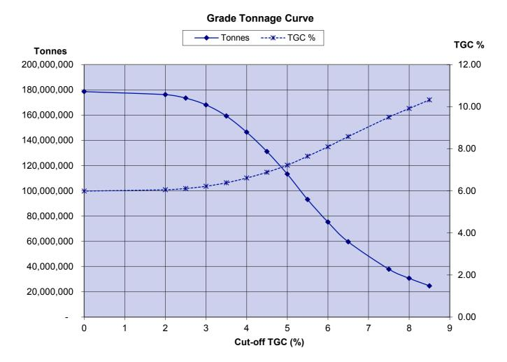
Figure 1: Grade Tonnage Curve – Measured, Indicated and Inferred
