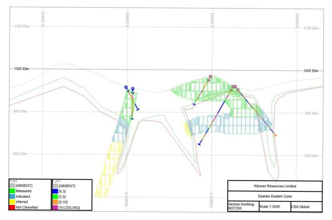
*Figure 7:* Cross section 9037200 through the East Deposit showing Measured, Indicated and Inferred Resource Blocks
