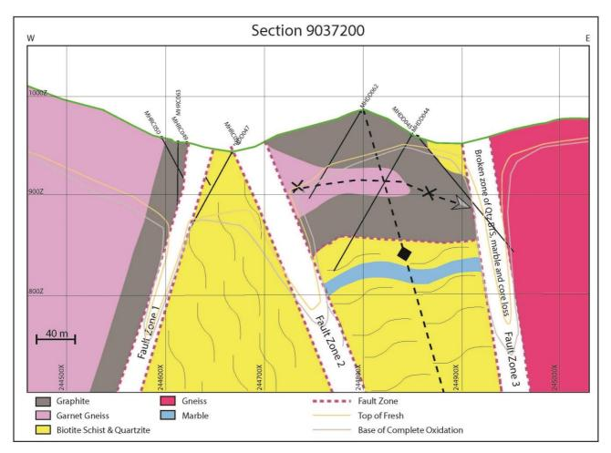
Figure 5: Cross Section 9037200N through the Epanko East Deposit
