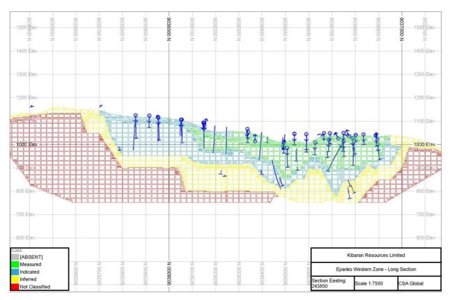
Figure 5: Long Section through the Western Zone showing the Measured, Indicated and Inferred Resource Blocks
