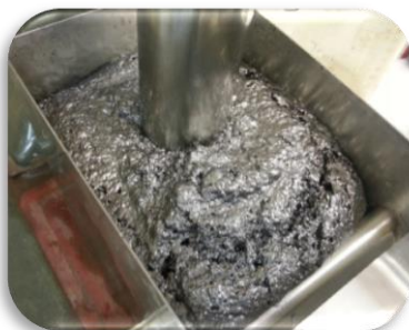
Figure 2: High Grade Concentrate - Final cleaner concentrate from an initial rougher cleaner test
