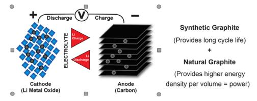
Figure 1 LiB Battery showing graphite anode (referenced and after Handbook on Rechargeable Batteries, 3<sup>rd</sup> Edition)
