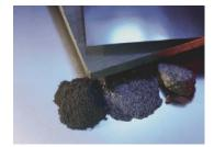
Ecophit® Expanded graphite manufactured into thermally conductive panels (Source: www.sglcarbon.com)
