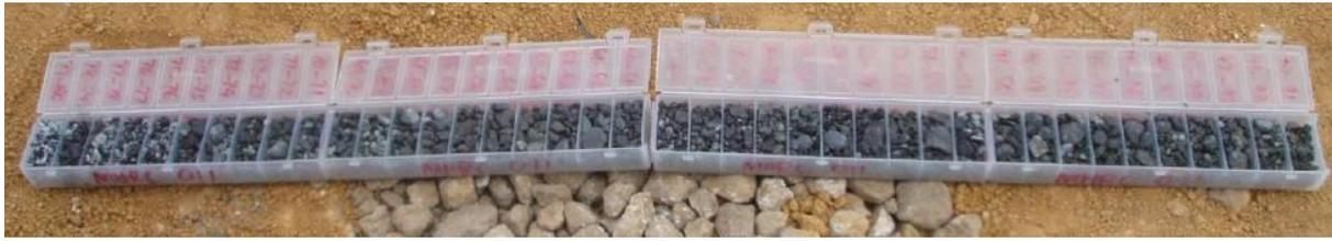
**Figure 4:** Chip Tray Record MHRC011, depth from 40 to 80 metres.
