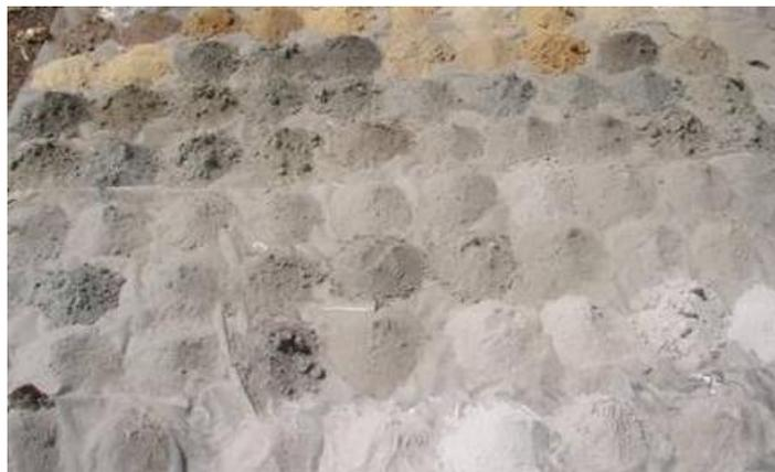
**Figure 1:** Site geological record at MHR008, showing the residual drill spoil. Each spoil pile represents one metre.
